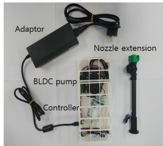
Fig. 1. Spraying tool to measure pesticide drift at wind tunnel.
