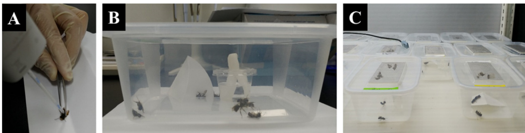
Fig. 1. The test supplies and set-up for acute contact toxicity tests: A, individual treatment (application) on the dorsal side of the thorax of solitary bees using the multipette M4 pipette; B, Groups of 10 bees were placed in the test cage with 50% sucrose feeders and a piece of filter paper; C, the overall testing setup.
