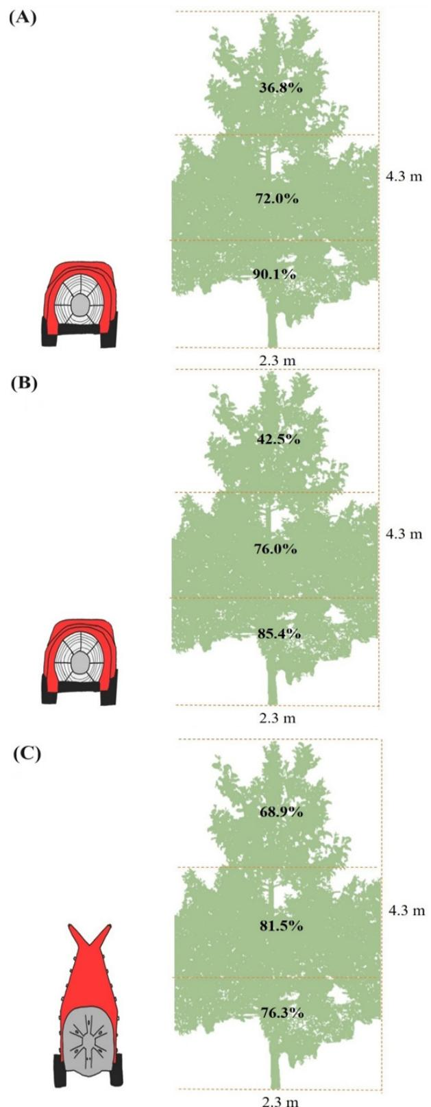
**Fig. 5** The difference in coverage rate by section according to the characteristics of the sprayer at 1,800 L/ha (A: axial; B: replacement nozzle; C: tower).
