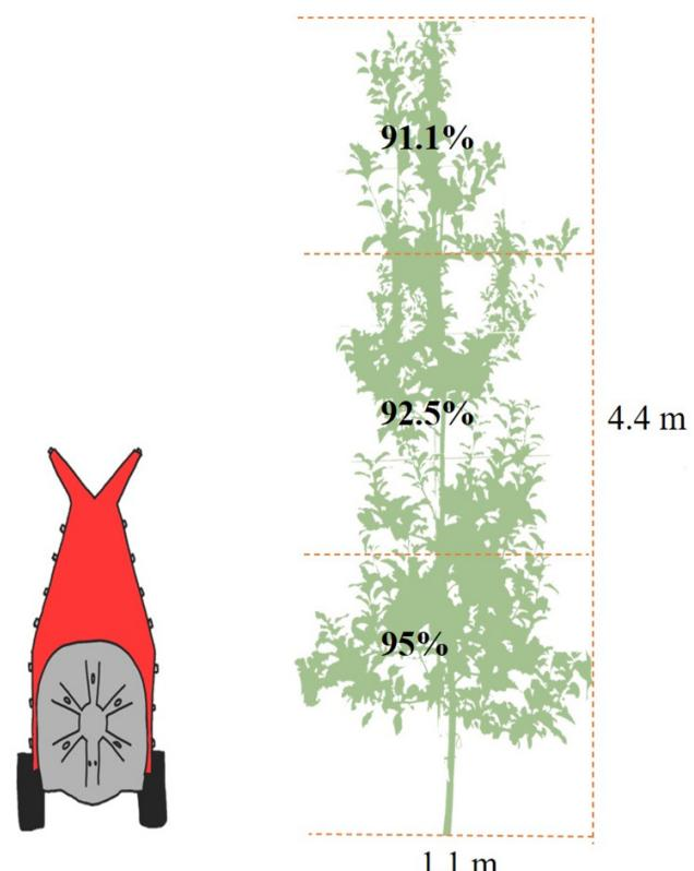
Fig. 6. The difference in coverage by tower sprayer at 1,800 L/ha in 3.6 × 1 m.
