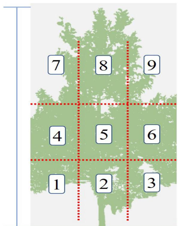
Fig. 4 Method of attachment of water sensitive paper.
