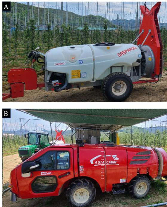
**Fig. 1** Air blast sprayers: (A) Tower type; (B) Axial type.
